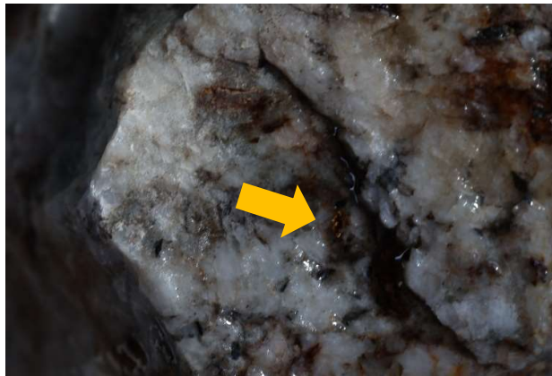
DRX_250811_007. Visible gold blebs in weathered sulphides in quartz veined grab sample. Field of view 9cm. (B, Figure 2)
