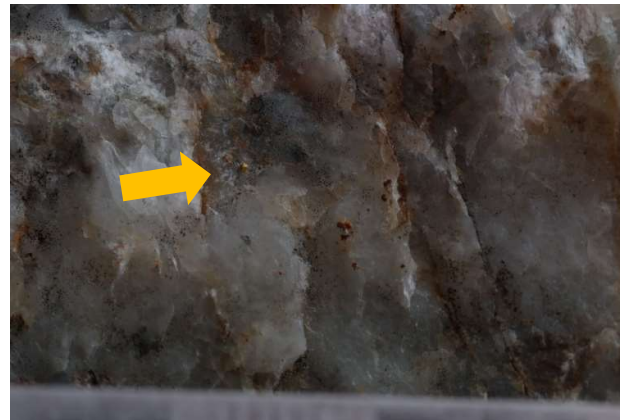
DRX_250811_007. Visible gold grains in quartz veining. Field of view 9cm. (B, Figure 2)
