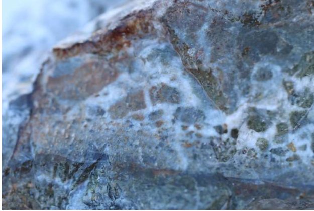
DRX_250811_006. Anomalous gold and high arsenic in annealed, carbonate-altered breccia. Field of view 9cm. (A, Figure 2)
