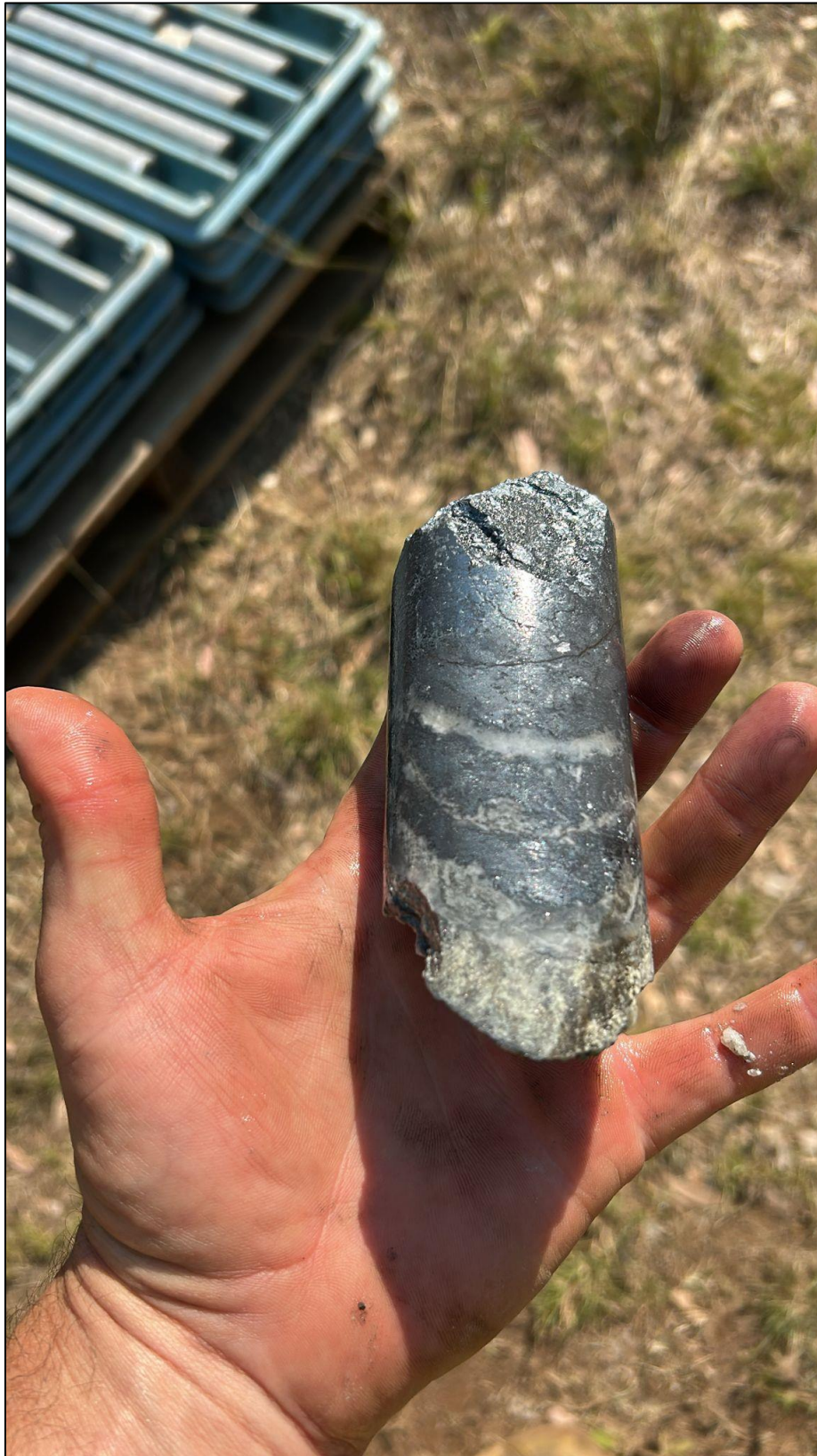
Figure 6: Stibnite and quartz veining from 42.0-42.1m downhole in Dart Mining's first drill hole at Coonambula (CBADD001). This is an example only and no sampling and assaying has been completed. Assay results will be provided when available*.
