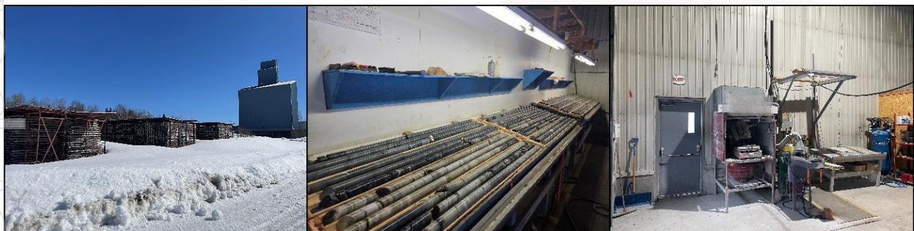
Figure 4 – Rouyn infrastructure (left to right) core racks & headframe, core logging station, automatic core saw
