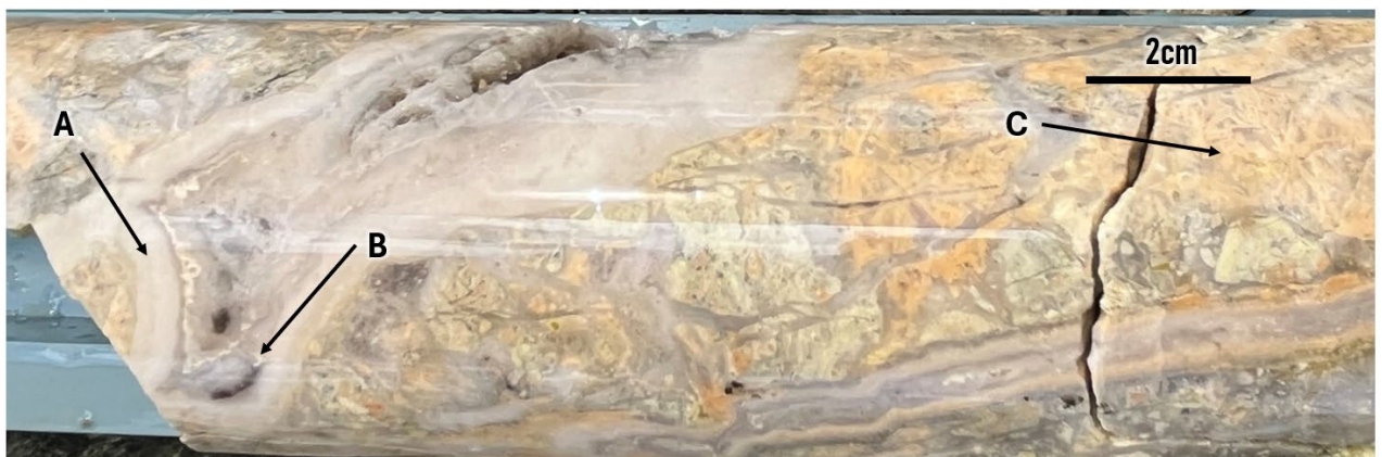
Figure 5: Cockade (A) sulphide banded (B) quartz-adularia (C) veining from A Vein in 25FCDD010.
