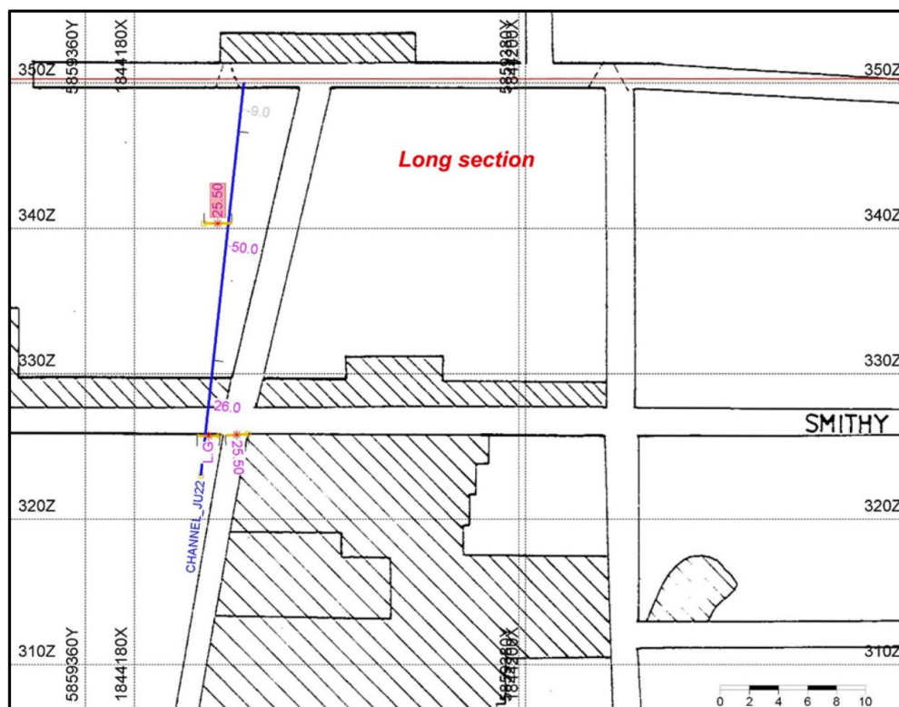
Figure 4: Channel_JU22: 23.0m @ 42g/t Au is a rise channel or vertical in the Long Section of the Jubilee mine
