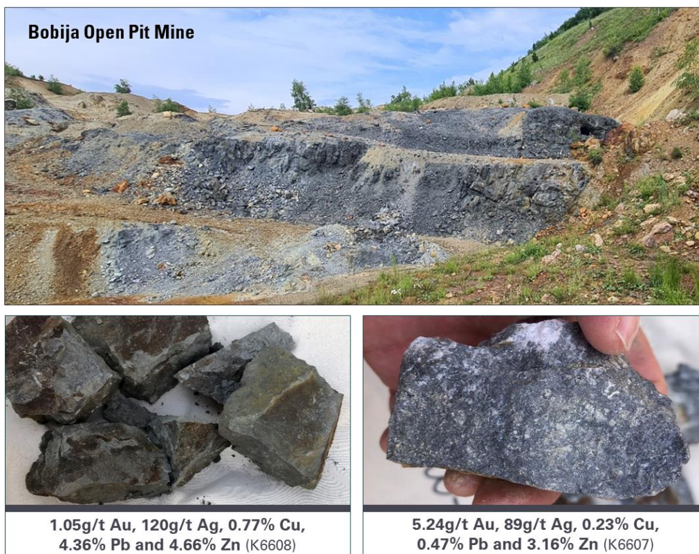
Figure 4: View of Bobija open pit mine with rock chip samples from the massive sulphide zone shown.
