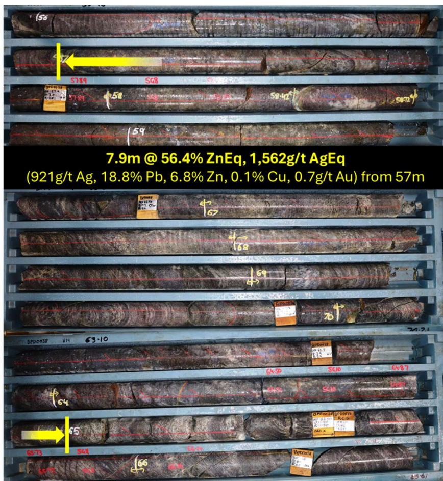
Figure 5 – Diamond drill core from BPD0038 within the Junction area of the Pinnacles Mine
