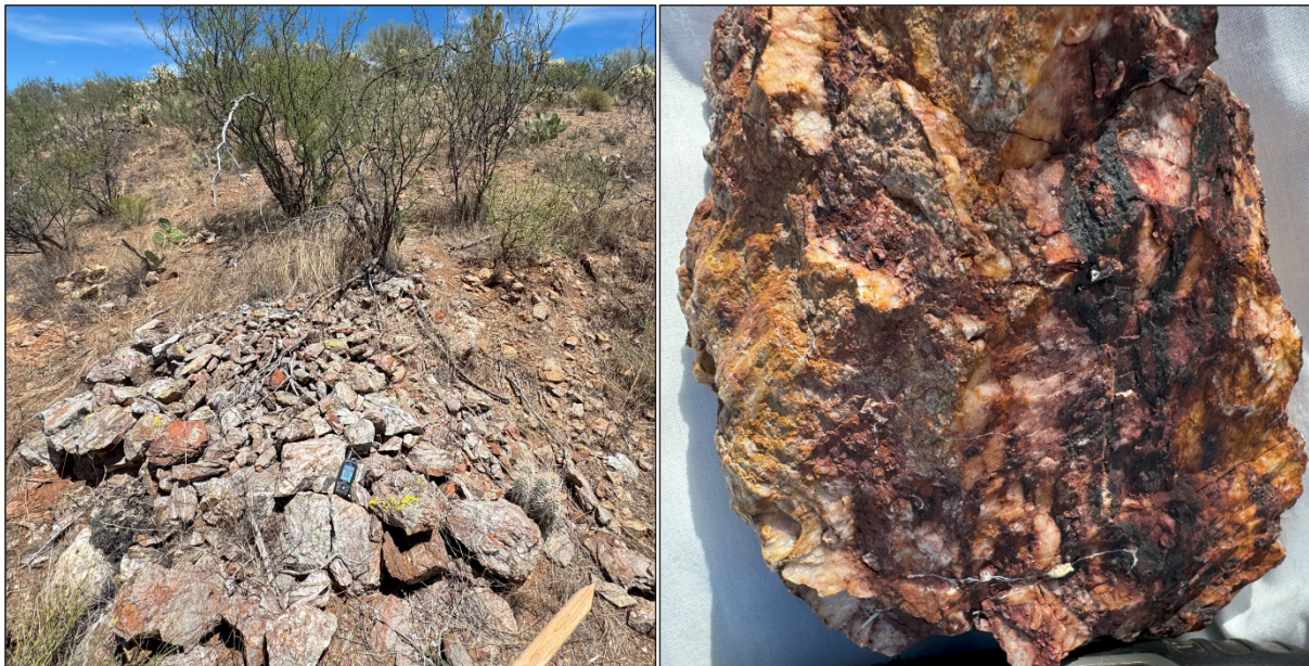
Figure 2: Aurora Prospect. Left: Sample 25RK001 29.3 g/t Au, 36 g/t Ag, 1.59% Pb. 2 Right: Sample 25RK002 11.2 g/t Au, 20 g/t Ag, 0.35% Pb. 2
