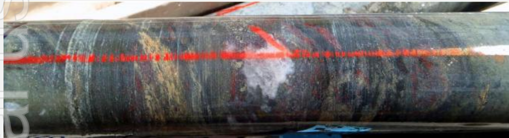
Veins of visible silver minerals (red-purple colour) from drillhole CMIPT077 from 174.4 m which assayed 1.8 g/t gold and 4,200 g/t silver over 0.3 metres 7
