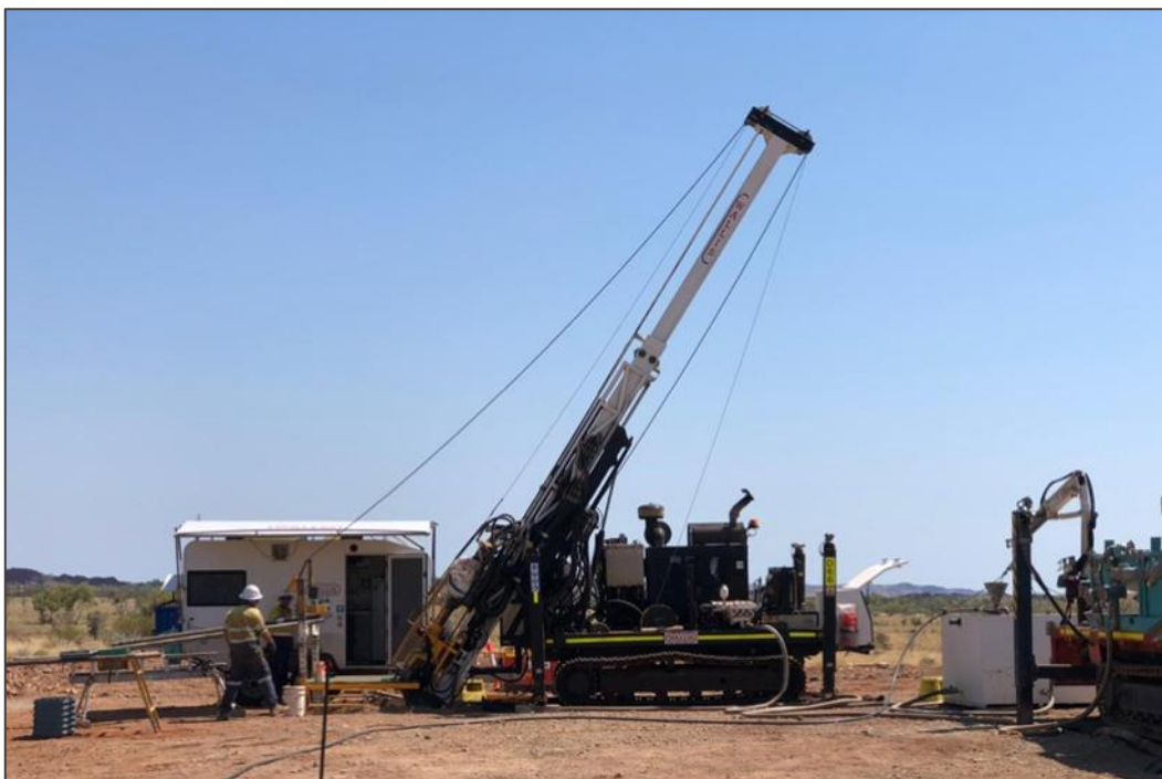
Figure 1: Diamond drill rig on site at Elizabeth Hill (Wallis Drilling), October 2025.
