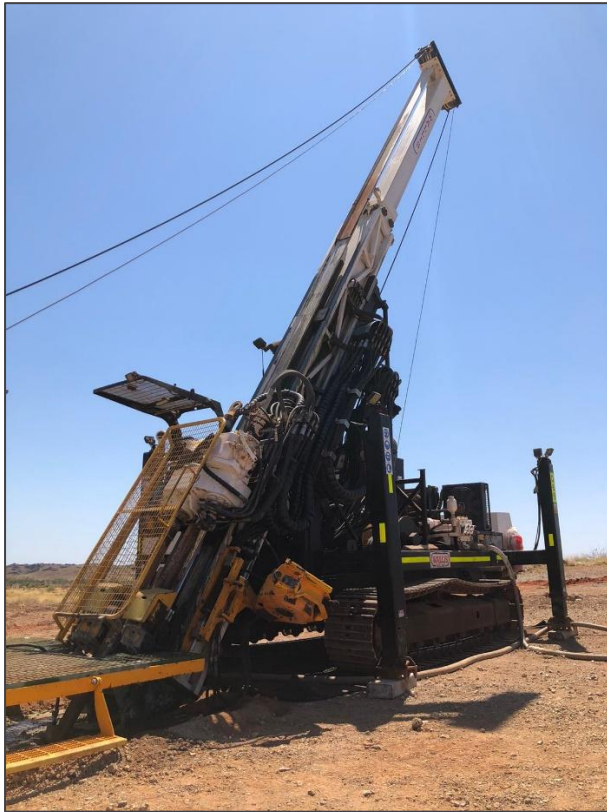
Figures 2 & 3: Diamond drill rig on site at Elizabeth Hill (Wallis Drilling), October 2025.
