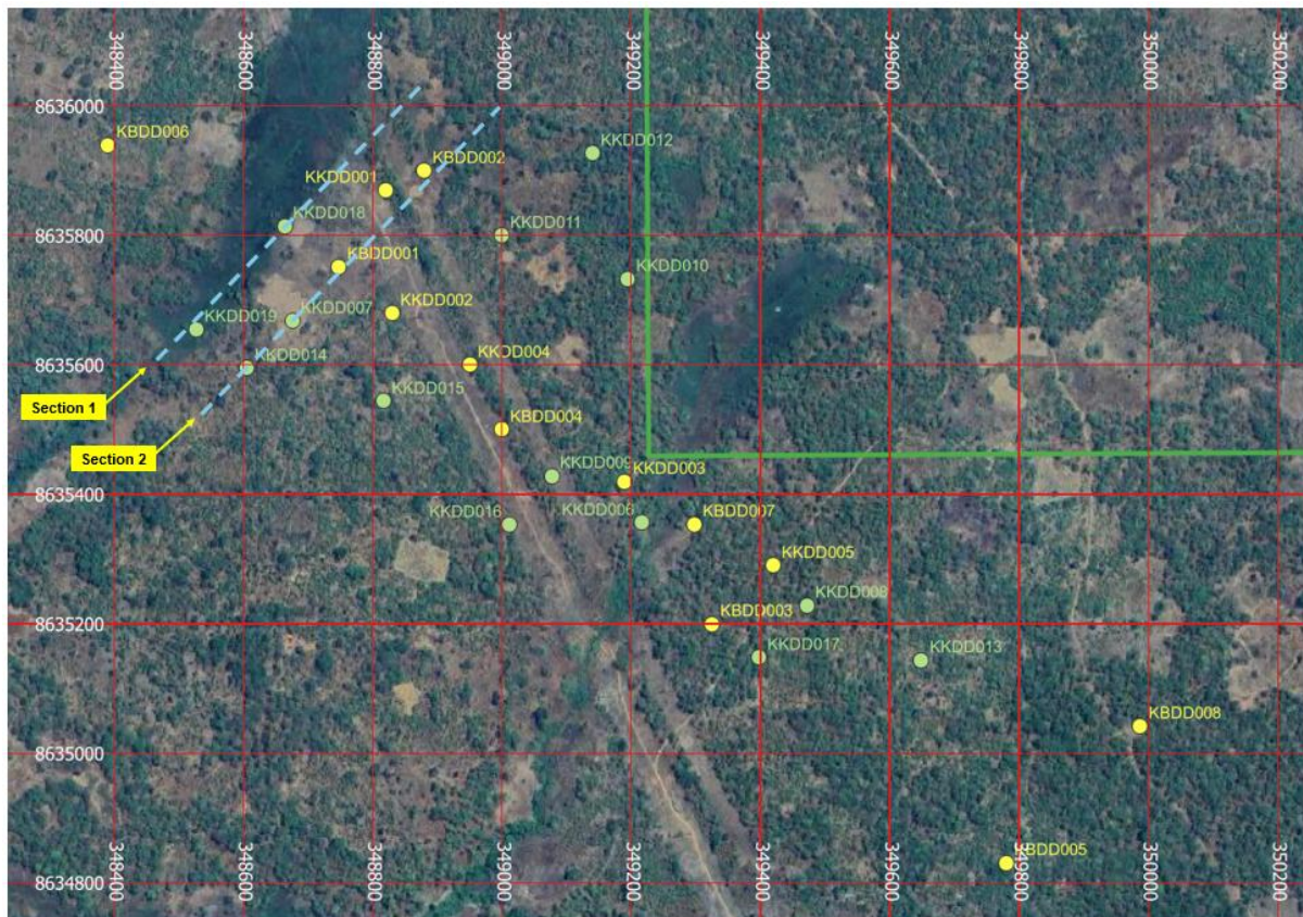
Figure 3. Kabikupa drill hole collar plan showing Prospect Phase 2 drill holes (green), pre-2025 holes (yellow) and oblique drilling cross sections described in this release (as dashed blue lines)
