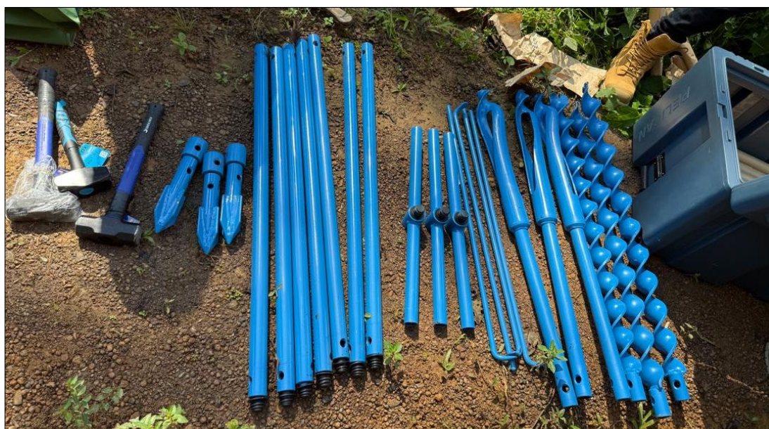
Figure 3: Hand auger equipment arrives on site.
