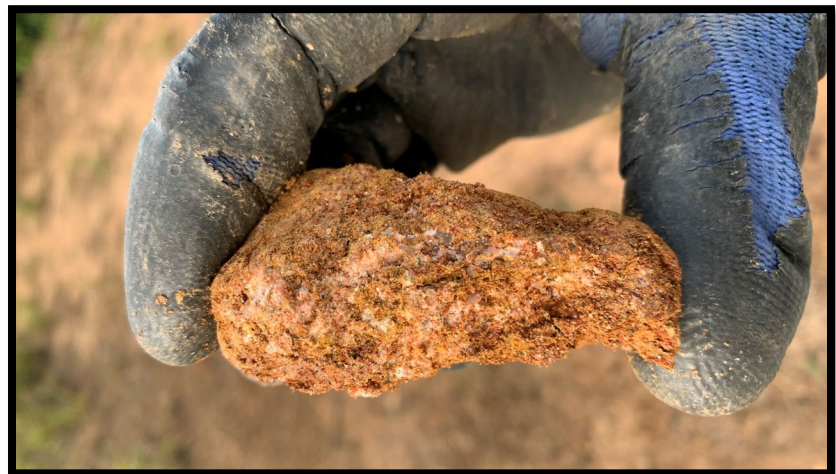
Above. Shallow mineralized interval from 2 to 3 meters depth in auger hole CAL-AUG-079 yielded 1,660 ppm TREO, with 34% MREO and 27% HREO (523ppm NdPr and 43ppm DyTb).
