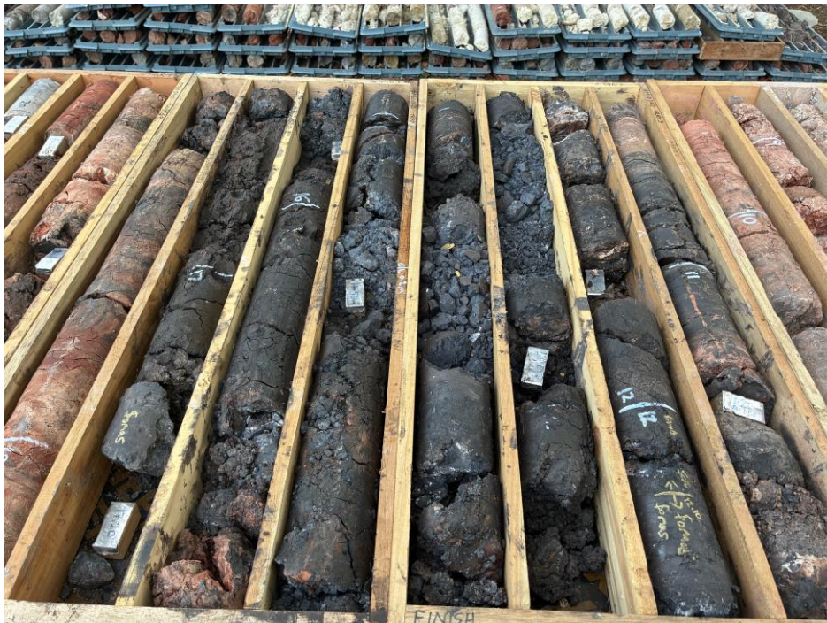
Figure 1: Primary and secondary manganese mineralisation in core from EMDD040. For visual estimates and visual estimates disclaimer please refer to table 1.
