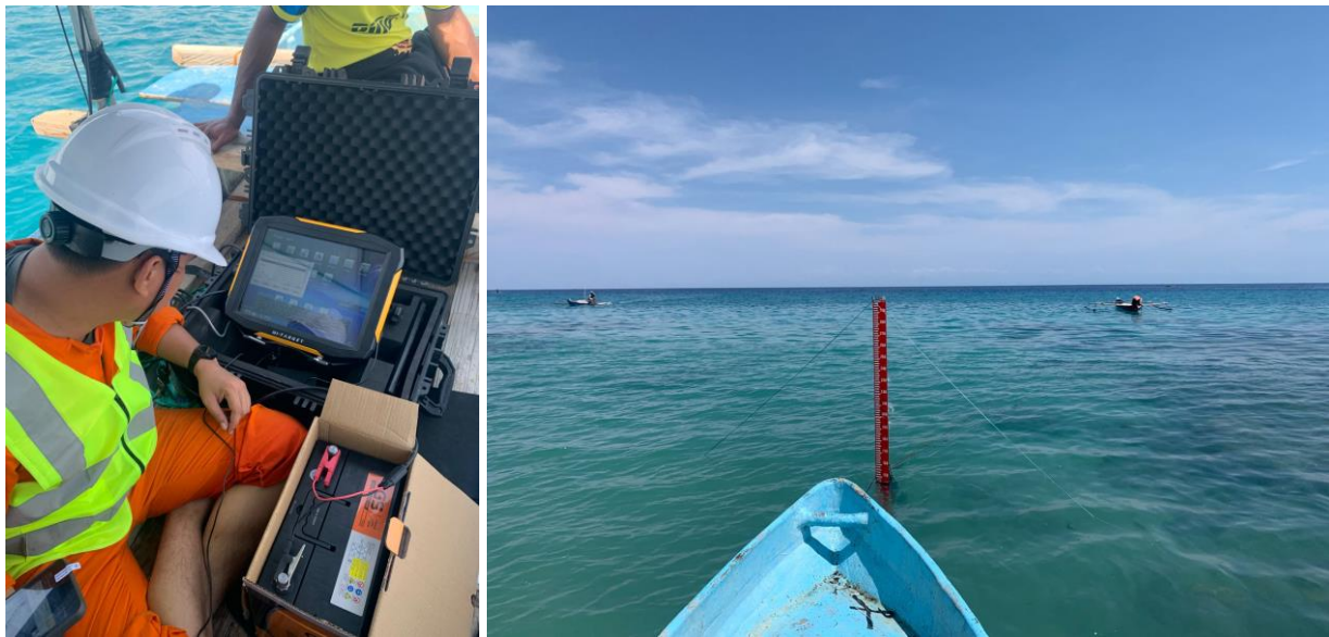
Figure 5: Bathymetric and Tidal Surveys underway at Werumata Limestone Project utilising support from the local fishing community
