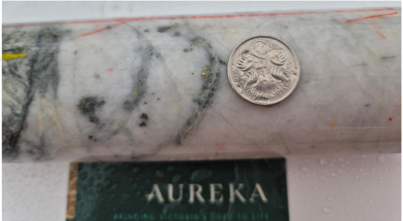
Figure 1: These 3 images show drill core containing visible gold from RD048 at 413m: 10m @ 12.1g/t Au from 413m (inc. 0.3m @ 183g/t Au from 413m and 0.3m @ 64.3g/t Au from 413.8m)
