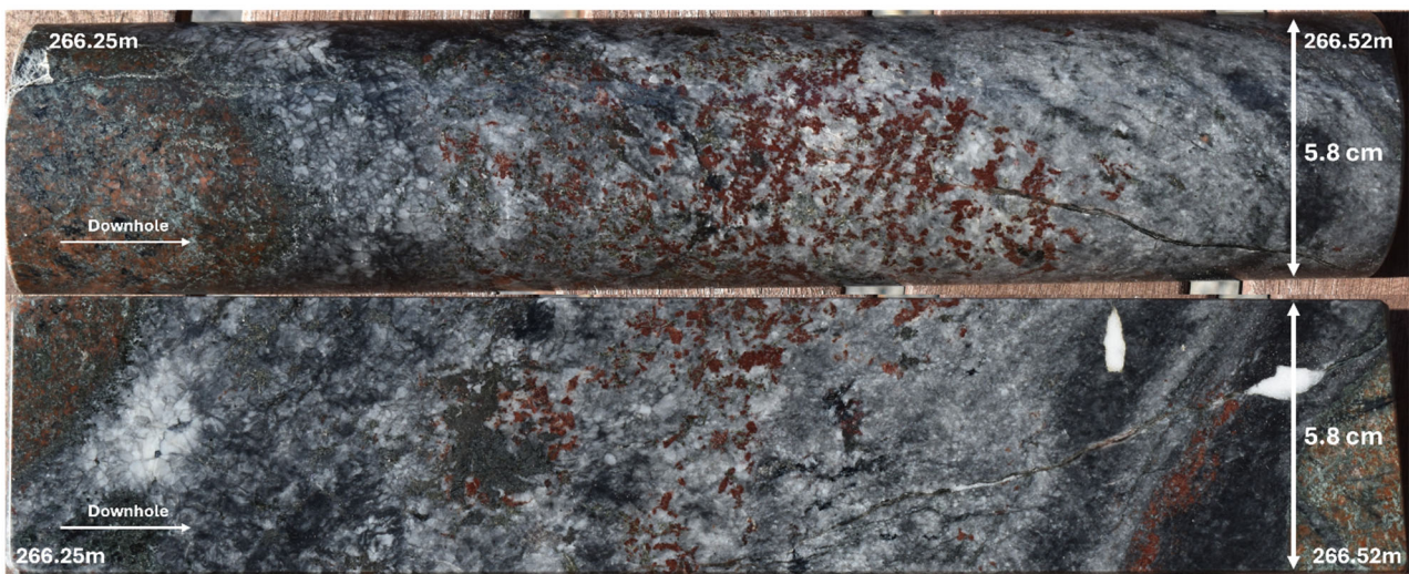
Photo 1 – EAL1370 – 266.25m – 266.52m – coarse red REE fluorocarbonate minerals in drillcore (1.1% TREO)
