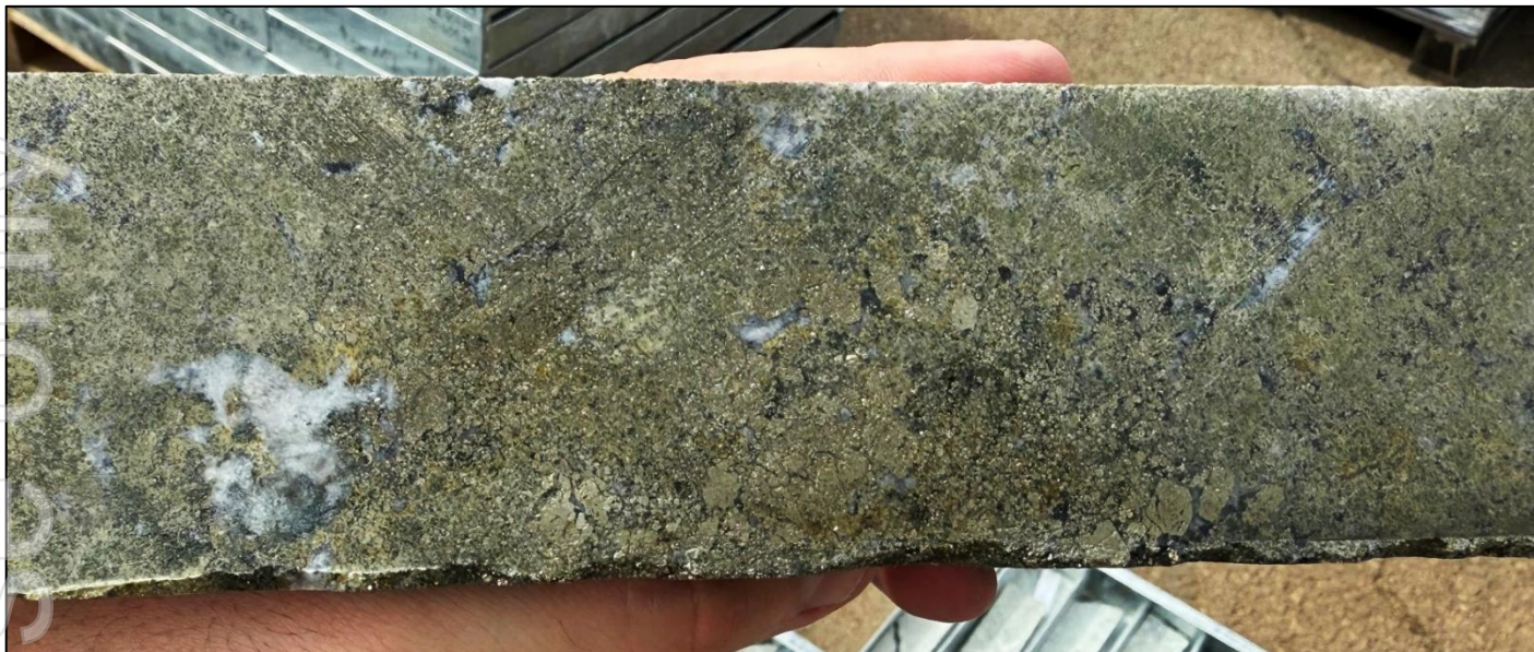
Figure 6. Core photograph of pyrite-rich skarn with disseminated arsenopyrite-sphalerite-galena from 292.2m to 294.2m in ZRSD25209 – assaying 4.6 g/t AuEq (4.6 g/t Au, 1.8 g/t Ag).
