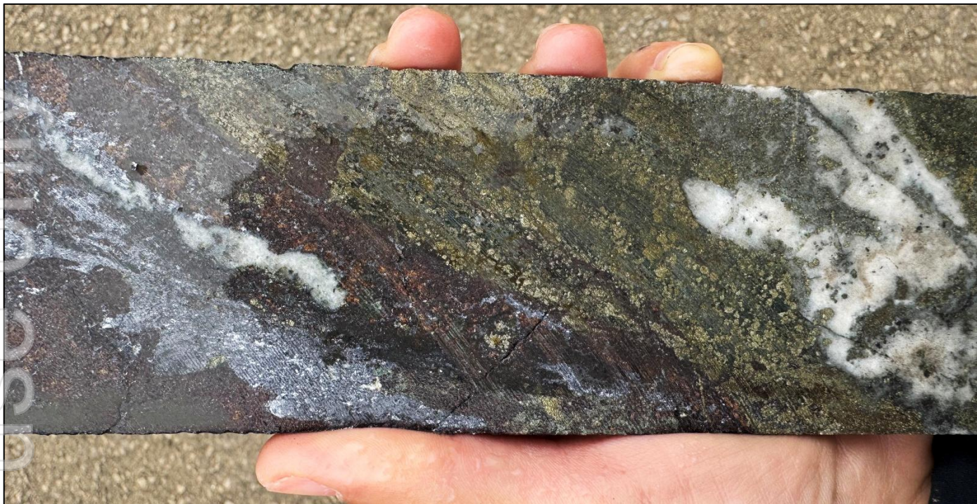
Figure 4. Core photograph of sphalerite-galena-arsenopyrite-pyrite skarn from the interval 344.7m to 345.9m in ZRSD25202 – assaying 8.3 g/t AuEq 2 (0.8 g/t Au, 6.1 % Pb, 6.8 % Zn, 98.7 g/t Ag).
