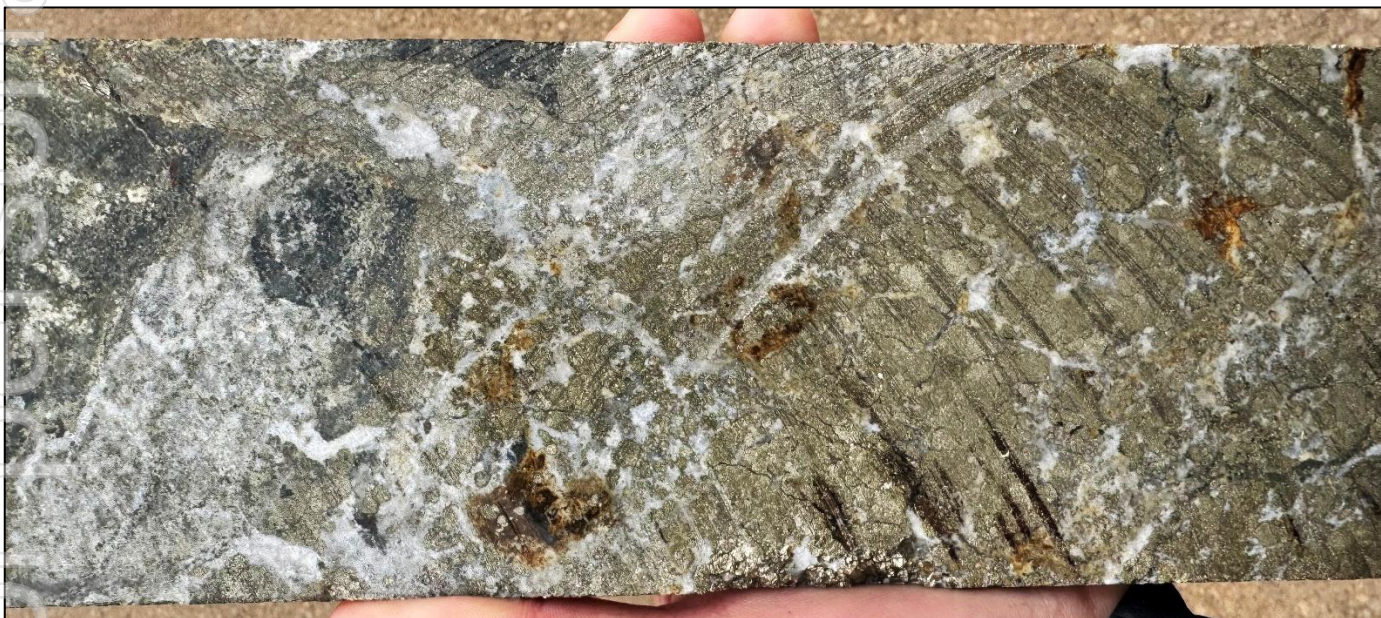
Figure 5. Core photograph of pyrite-rich monomictic andesite breccia with strong silica alteration from 279.0m to 280.2m in ZRSD25205 – assaying 10.8 g/t AuEq 2 (10.7 g/t Au, 2.7 g/t Ag).
