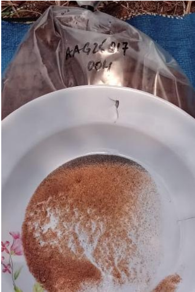
Figure 1 (Left): A pan showing heavy mineral concentrate (HMC) from hand auger drilling hole 17 in alluvial material within Adriano (11002L).
