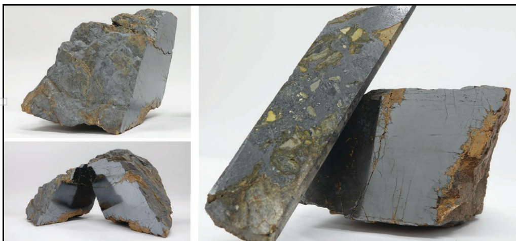
Fig 1: Massive stibnite from surface trenching (top: trench 25NWTR005; bottom: samples from trench 24NWTR004 assaying 3m @ 50.26% Sb and core from 25TCDC004 up to 24.9% Sb). Previously reported results (ASX: 12 Feb, 30 May, 15 Sept, 7 Oct 2025).
