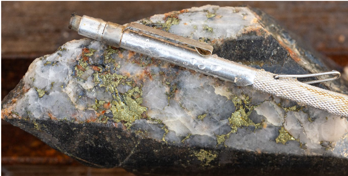
Figure 2. Coarse grained chalcopyrite in quartz veining at down-hole depth of 14m hosted in a 2.7m interval of potassic altered volcanoclastic sediments. Visual estimates of chalcopyrite abundance in this 2.7m interval are between 0.6% and 0.9% by volume, representing indicative copper grades between 0.2% and 0.3% Cu.
