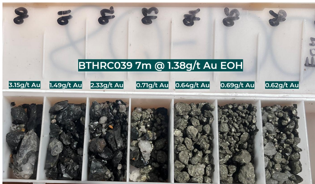
Figure 7: Photo of BTHRC039 chip tray with 1m intervals and gold grades from 89m to 96m EOH 1 . Geology changes from chert and quartz veining, into quartz veining and massive pyrite toward end of hole.
