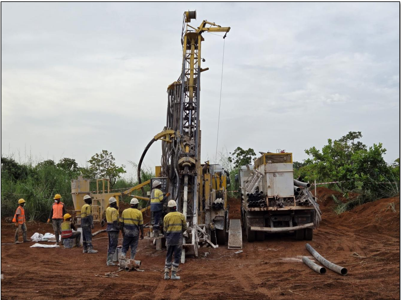
Figure 1 – RC Drilling underway at the Dadjan Gold Project Guinea, the first recorded drilling on the permit, with 50 years of recorded artisanal mining.
