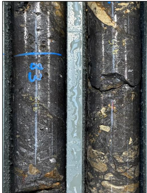
Photo 2. 19.61% Sb over 2.4m from 82m within 9.92% Sb over 4.8m from 81.5m (MAG010)
