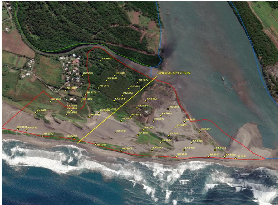
Figure 3 - Kulukulu South area, indicating the location of the cross-section shown in Figure 4. Also note the sand and gravel deposits filling the Sigatoka riverbed that will be dredged during the Desilting Project.
