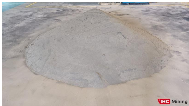
Plate 1 – “Run of mine” magnetite bearing construction sand sample from Kulukulu South resource area
