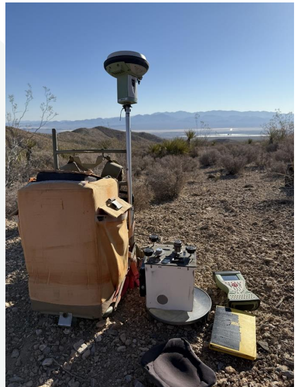
Figure 1: Field crew conducting ground magnetic and gravity survey at Desert Star Project
