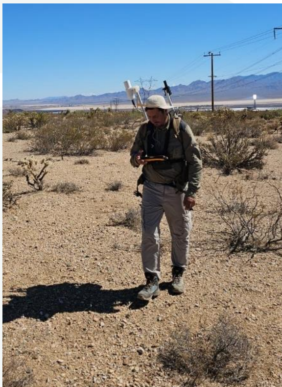
Figure 1: Field crew conducting ground magnetic and gravity survey at Desert Star Project
