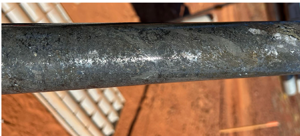
Figure 1: Core from drillhole EHDD25001 (~240m depth) showing semi-massive sulphide mineralisation (pyrite-pyrrhotite-boulangerite ( Pb_5Sb_4S_{11} )) within a zone of quartz-sulphide stockwork veining. Sulphides in this interval constitute ~50% of the rock shown. Assays are pending for this interval.
