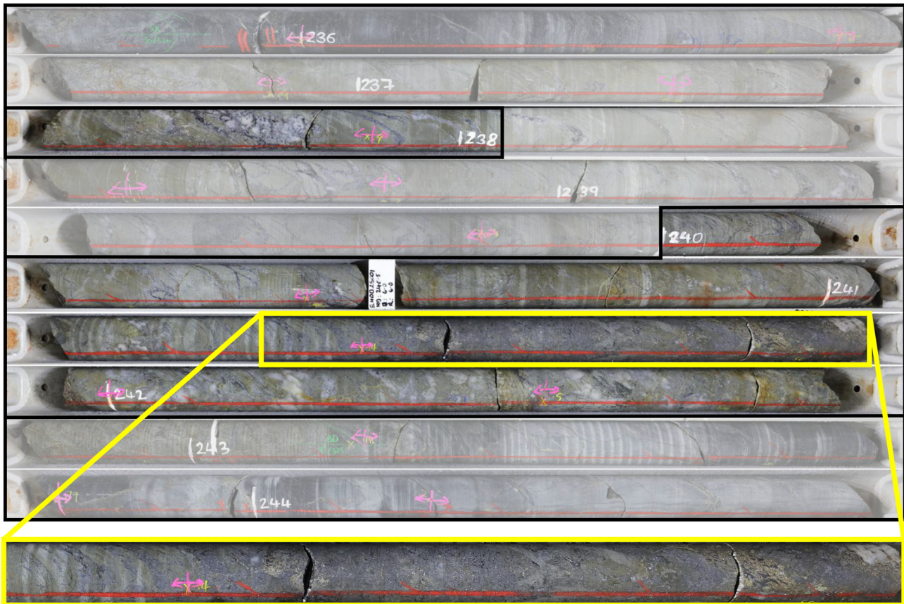
Figure 5: Photo of mineralised zones from EHD25001, with a close-up of a zone of boulangerite ( Pb_5Sb_4S_{11} )-pyrite-quartz veining. The intervals highlighted show a series of quartz-boulangerite stockwork veins that returned elevated Sb results from Truescan XRF scanning. Assays are pending for this interval. Note: visual estimates of mineral abundance should never be considered a proxy or substitute for laboratory analyses where concentrations or grades are the factor of principal economic interest. Visual estimates also potentially provide no information regarding impurities or deleterious physical properties relevant to valuations.
