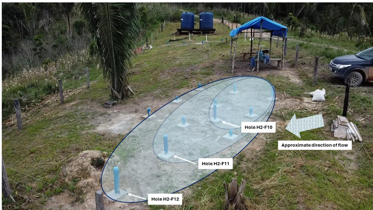
Figure 4. Field pilot trial and setup showing distribution of monitoring holes H2-F10, H2-F11, H2-F12. Rings indicate approximate area of leaching influencing grades received from the PLS, with H2-F10 being the smallest leaching area.
