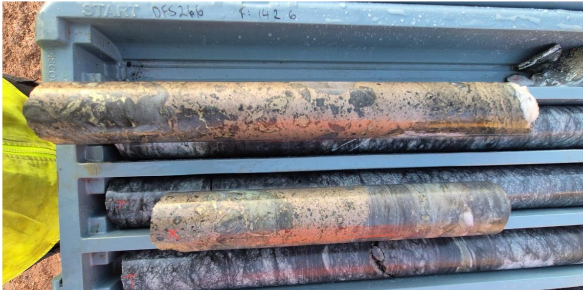
Figure 1 - Mineralised Interval from infill drill hole DFS266 – 1.4 metres at 51 g/t gold from the 2140 lode consisting of massive pyrite-chalcopyrite in a silica matrix with visible gold.
