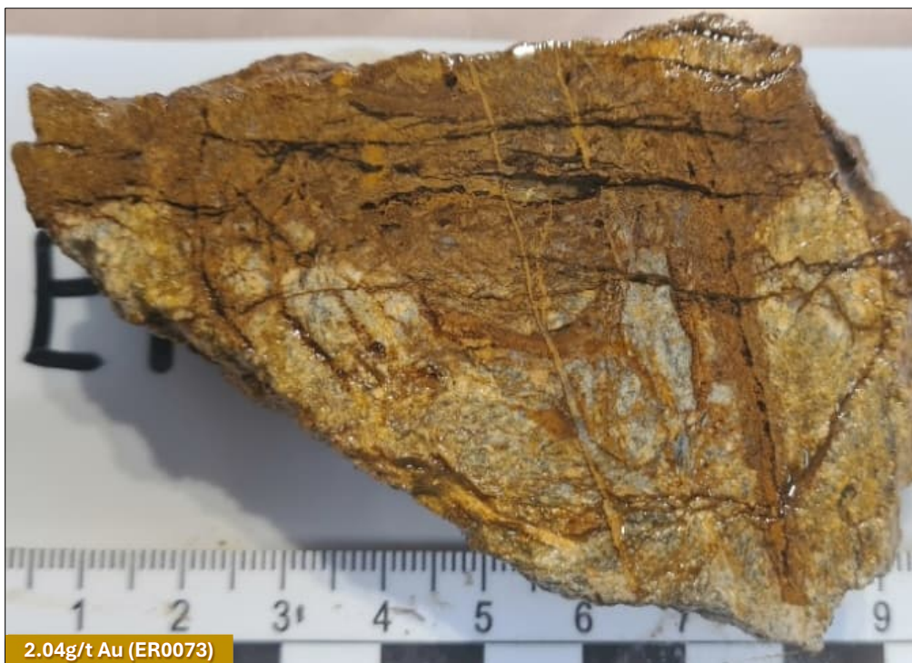
Photo 4. 2.04g/t Au rock chip sample from mullock pile at Borah of gossanous, quartz-sericite-limonite altered, medium grained granite, with stockwork limonite \pm quartz veins with boxworks after sulphides. Numerical units on scalebar are centimetres.
