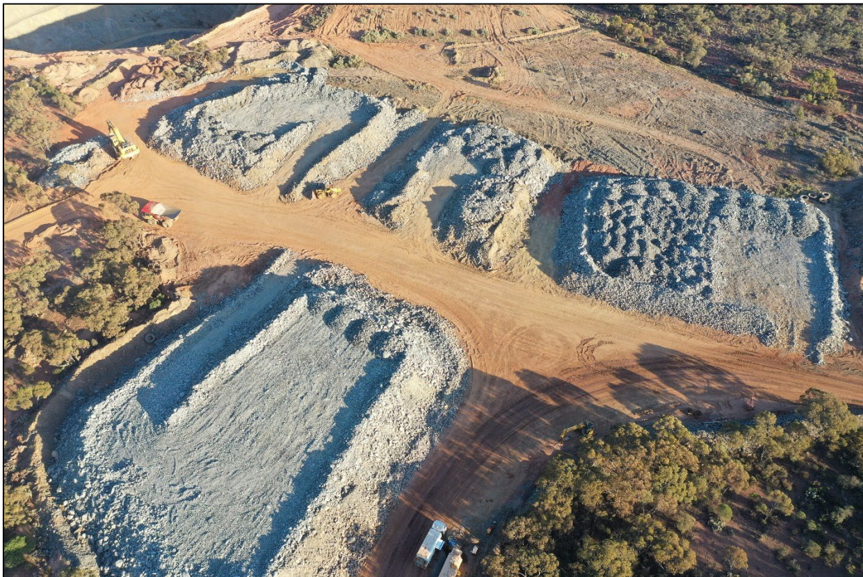
Figure 3: Ore on the Phillips Find ROM pad.
