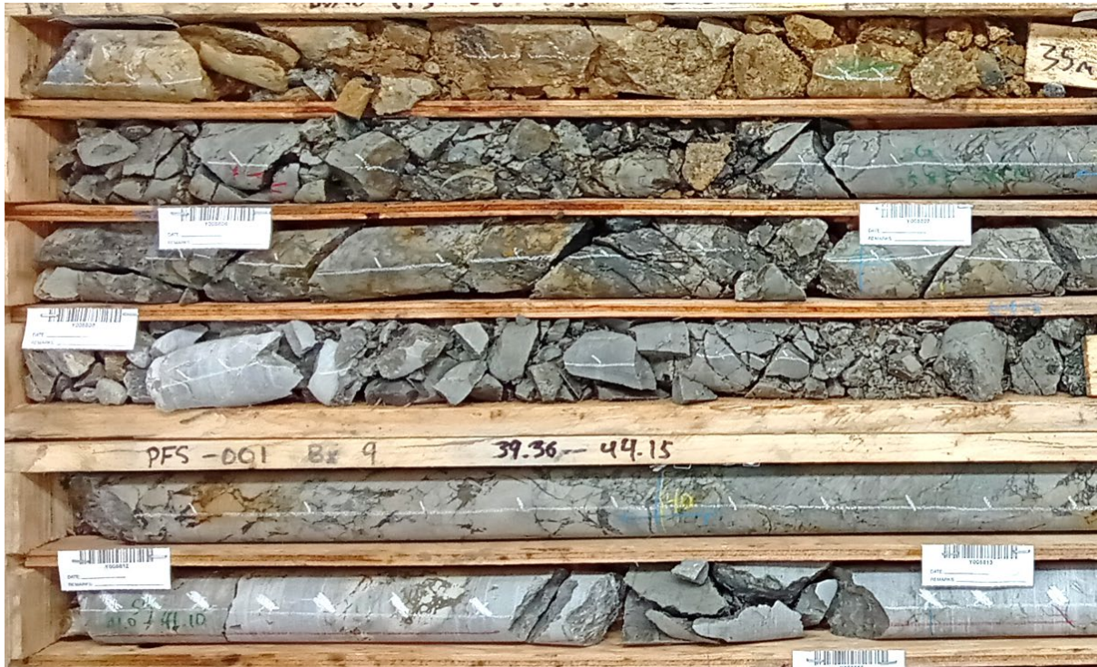
Figure 2: Dense breccia and semi-massive visual chalcocite (dark grey mineral) in drill hole PFS-001 (33.4-40.5m downhole). This interval assayed at an average grade of 2.2% Cu, 12g/t Ag.
