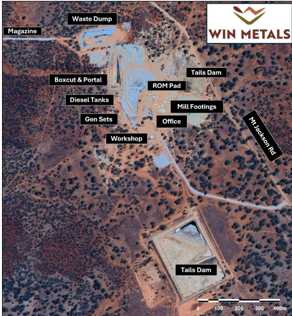
Figure 4: Radio Mine Site Layout and Infrastructure
