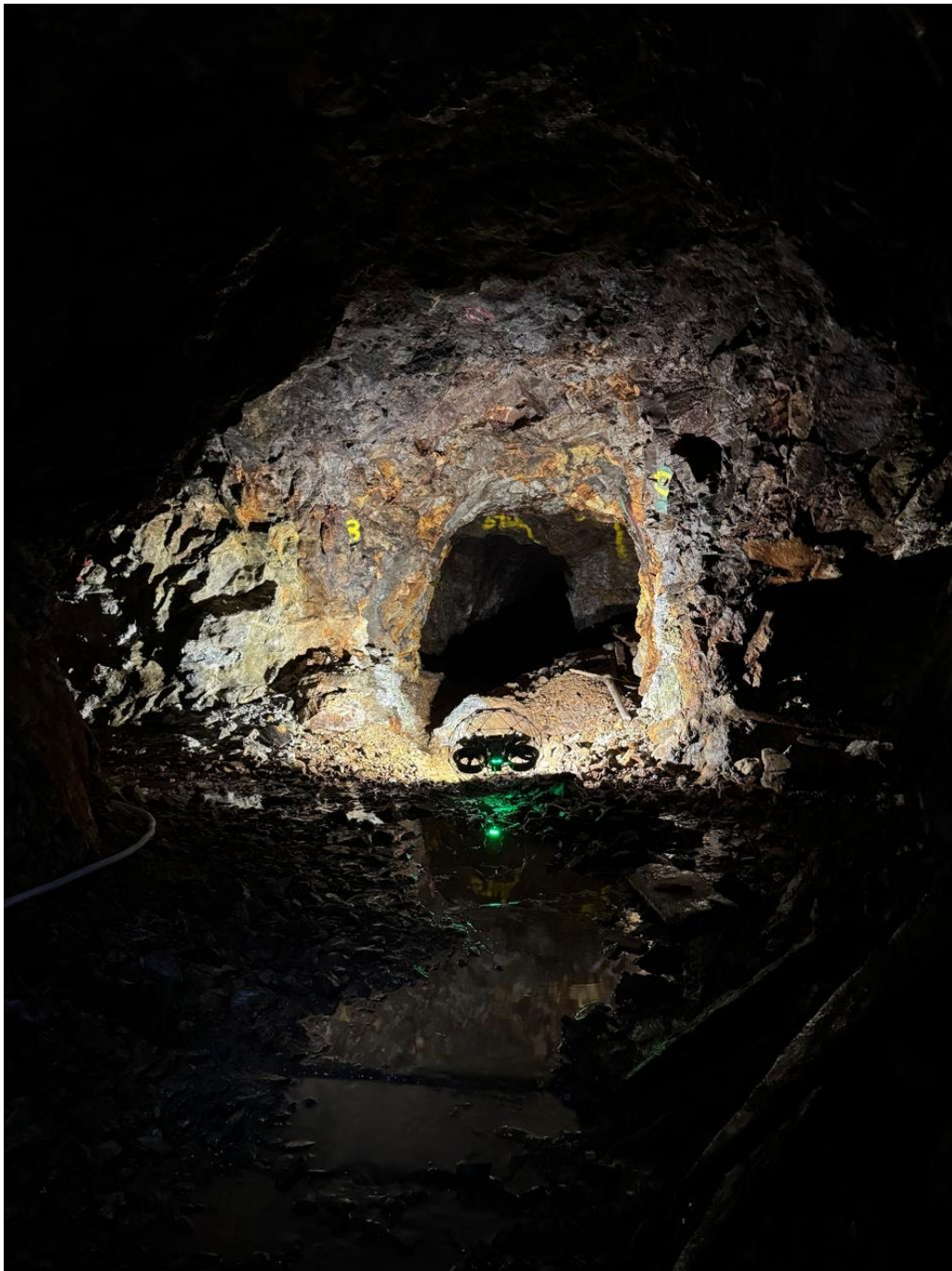
Photograph 2 Drone flying deep in Adit 117, surveying the adit walls.
