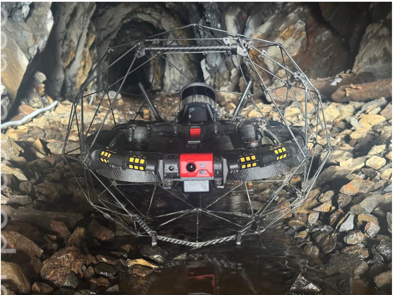
Photograph 1 Elios-3 drone setup at the adit mouth, preparing to be flown.
