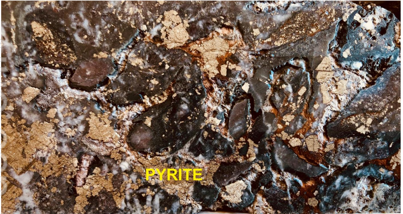
Figure 2 Epithermal breccia mineralisation (79.4m, Drill Hole 25L1MP3DD001)
