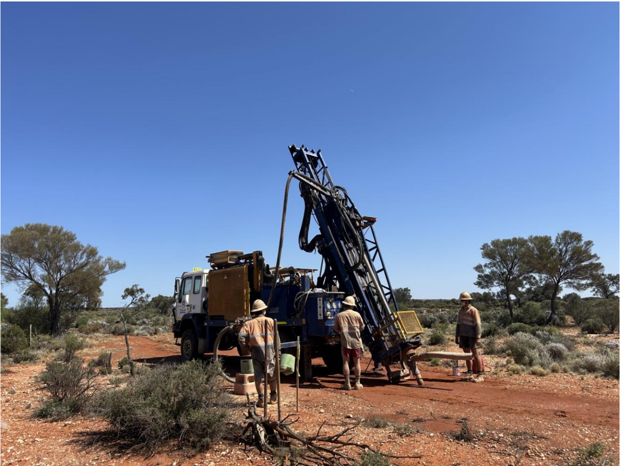
PHOTO 3. AIRCORE DRILLING AT BRANCHES PROSPECT OCTEBER 2025
