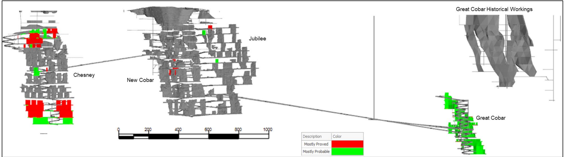
Figure 7: Long section facing west of the New Cobar Mine showing Proved (red) and Probable (green) Ore Reserve classifications.
