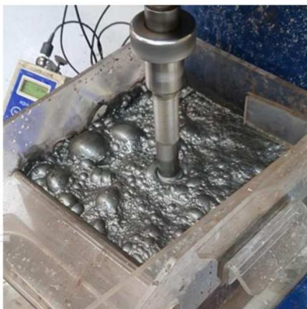
Figure 4 – Transitional Ore Flotation Test ( left) and concentrate (right)
