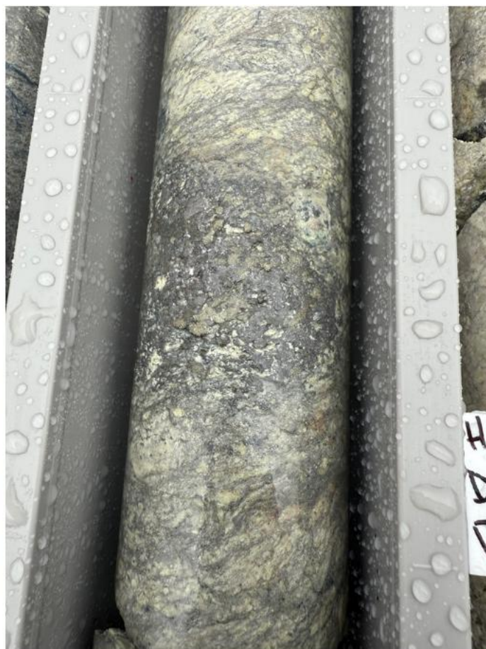
Sulphide bleb (arsenopyrite-pyrite) in kaolin-sericite alteration at 134m in WBR039
