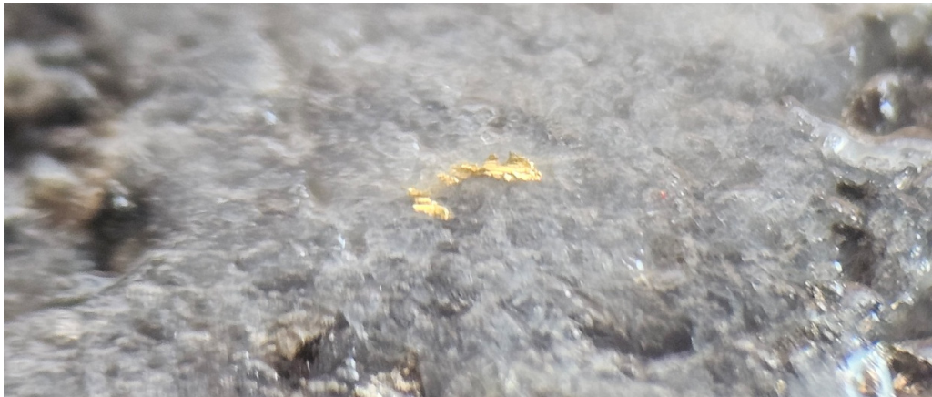
Figure 1. Visible gold in drill core from diamond drill-hole 25XCDD002 at 150.05m down-hole, the second instance of visible gold at the Martin Prospect. Field of view width 5mm, refer Table 1 and Figure 2 for additional information.
