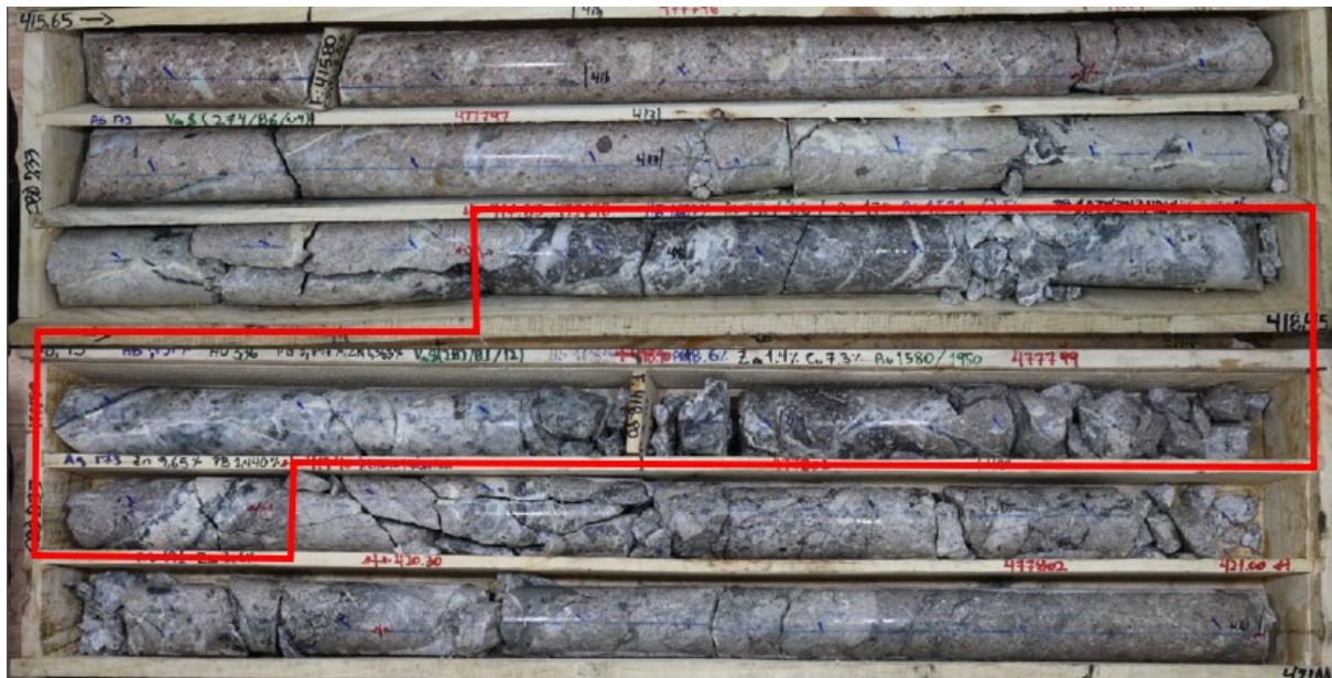
Figure 4. CBD233 Hanging wall mineralised quartz breccia, 1.5m @ 3,168 g/t AgEq from 417.9m to 419.4m.
