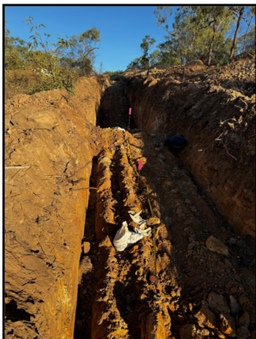
Figure 2. Channel rock chip sample 102554 (3m length in foreground) was collected along the bottom of Costean 1 at Muscleville and returned 3m @ 2.37 g/t Au within a 4m wide breccia zone that assayed 2.07 g/t Au. This structurally controlled zone of gold-silver mineralisation trends northerly along the sheared contact separating the Chillagoe Formation from the Hodgkinson Formation in the east. Outcrop grab (SampNo 102551) of silicified breccia adjacent to the costean at this location assayed 6.48 g/t Au, 38.4 g/t Ag, 10.3% As and 0.44% Sb.
