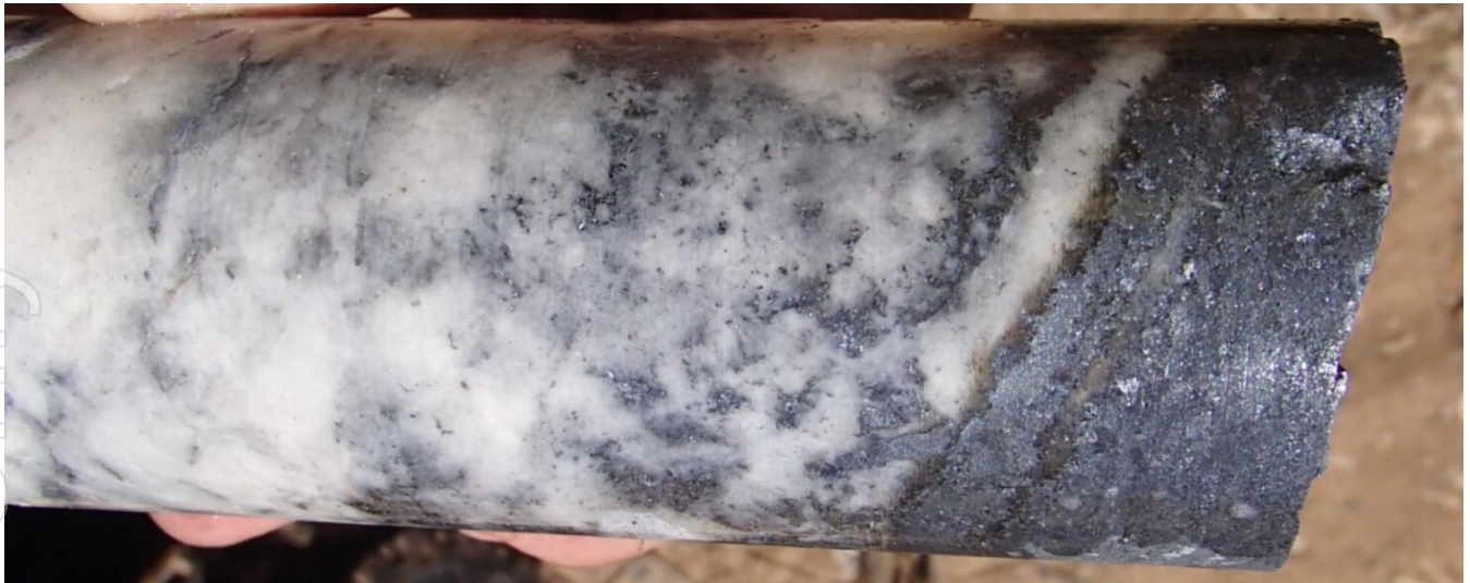
Figure 5: NQ drill core from 131.45m depth from CBADD003. Massive stibnite on the right of the core from 131.6m, with quartz and stibnite to the left. Detailed logging and sampling are underway, assays expected in November.
