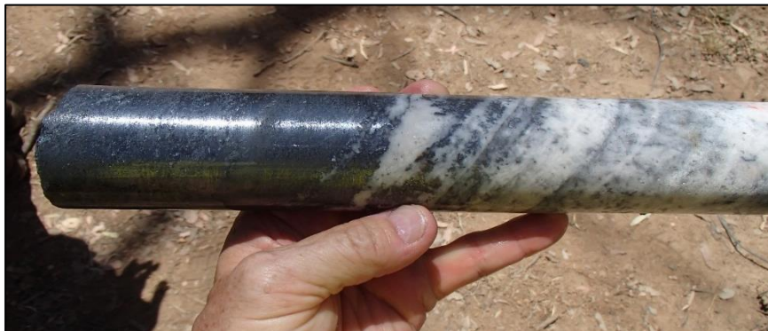
Figure 1: Wet drill core from 131.65m depth from CBADD003. Massive stibnite on the left of the core, with laminated quartz and stibnite to the right. Drill core contains an estimated 0.2m with 95% Stibnite, with a surrounding 0.9m of 10% Stibnite in Quartz. Logging is underway, with sampling and the return of assays expected in November.
