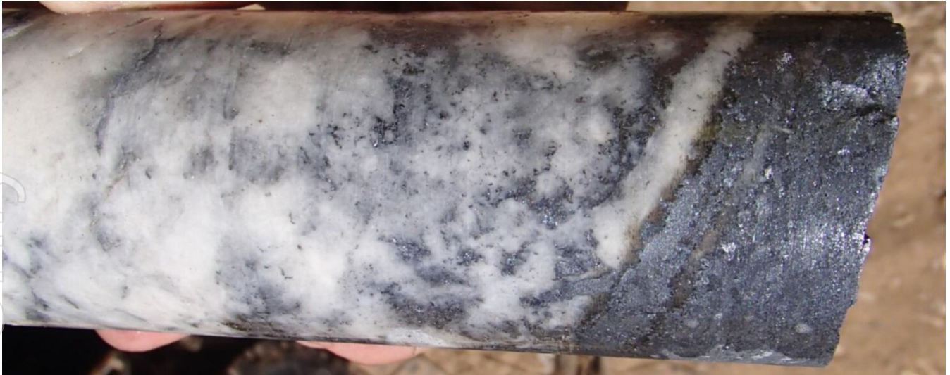
Figure 5: NQ drill core from 131.45m depth from CBADD003. Massive stibnite on the right of the core from 131.6m, with quartz and stibnite to the left. Detailed logging and sampling are underway, assays expected in November.
