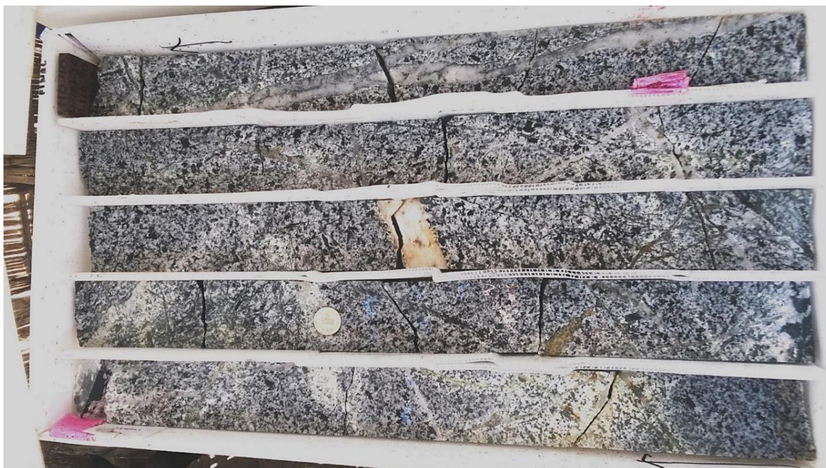
Figure 9: Drill core from historical hole COP14-06 showing quartz veining, copper sulphides and stockwork. Core shown commences at a depth of 122.00 metres and ends at 125.00 metres. Associated drillhole assay results: 175.4 metres @ 0.28% Cu, 0.012% Mo and 1.3 g/t Ag (from surface) inc. 91.2 metres @ 0.33% Cu, 0.007% Mo and 0.8 g/t Ag (from surface) (Table 1).
