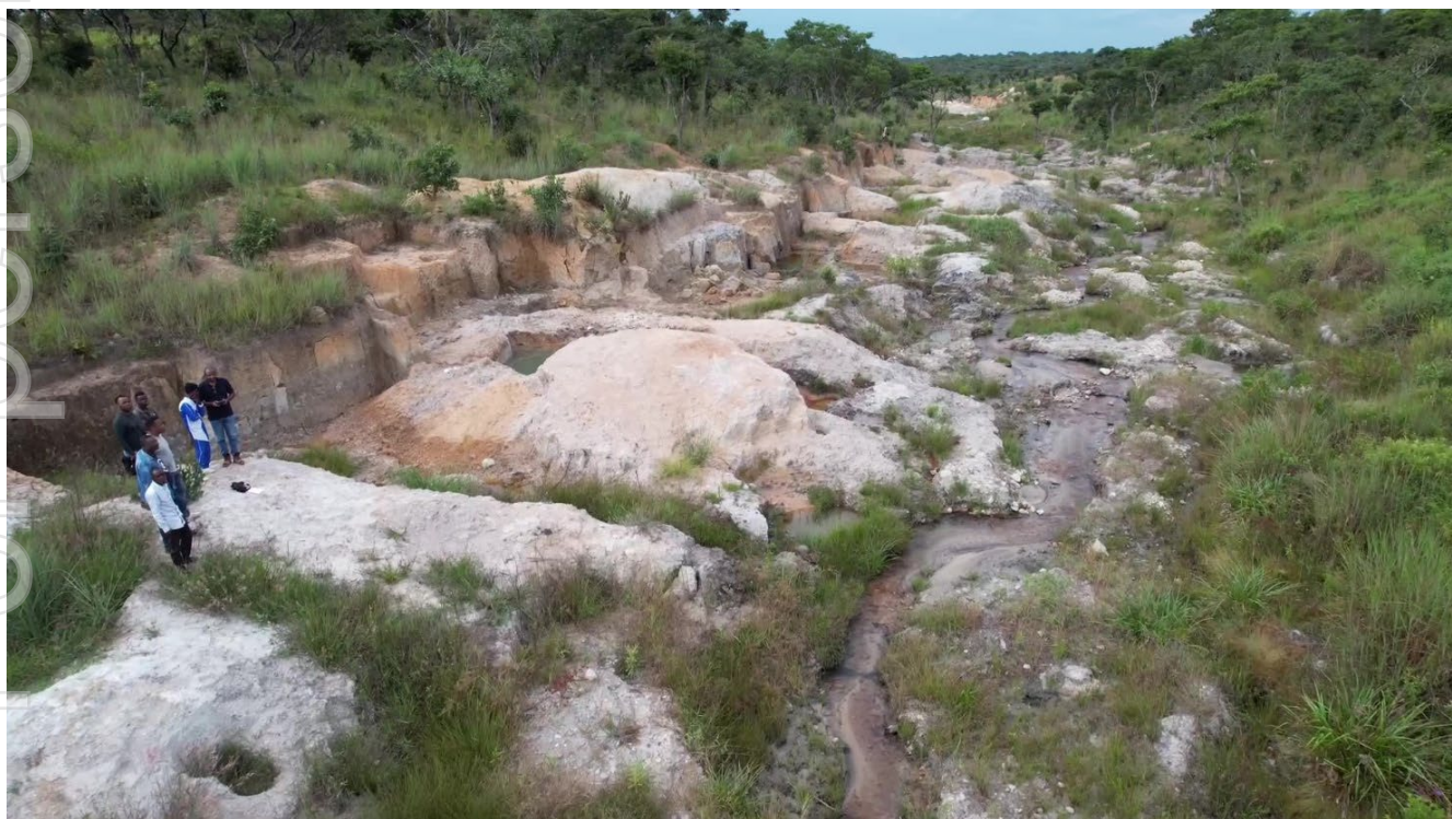
Figure 4. A seasonal river at Longundo . Garimpo pits are dug to access gold-mineralised gravel beds at the base of recent alluvial sediments
