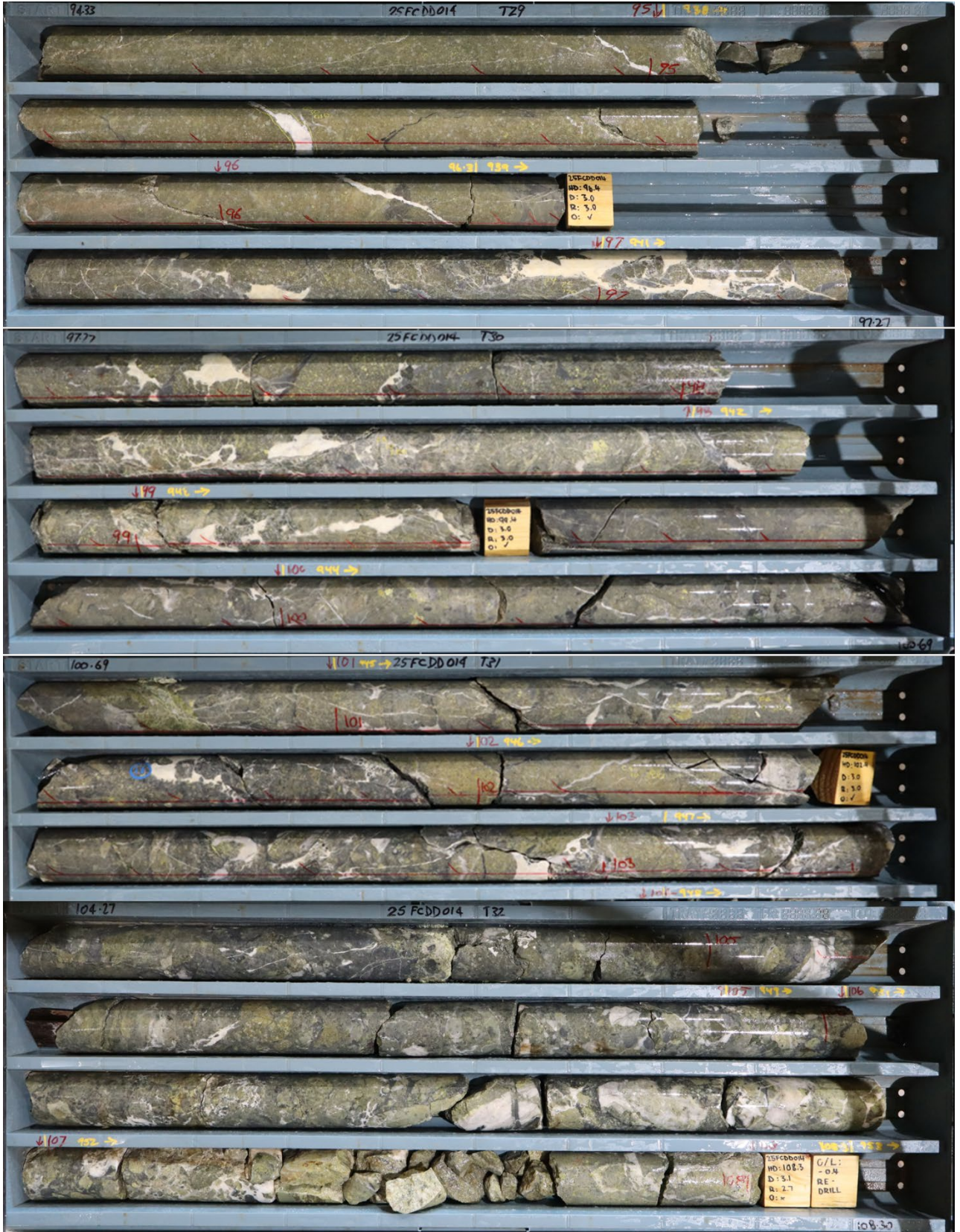
Figure 3: Breccia observed in 25FCDD014 from 96.4m to 108.5m.
