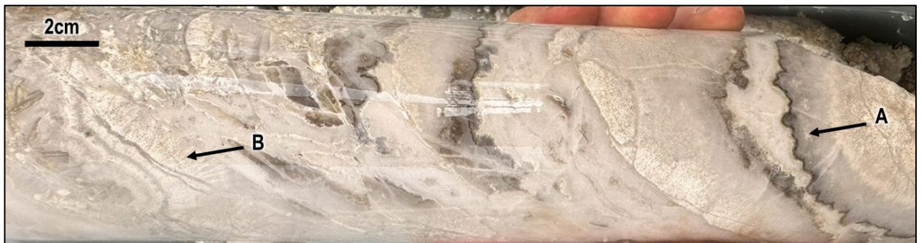
Figure 1: Marcasite colloform (<1% vein fill, A) within colloform – crustiform, quartz – adularia (B) from from high-grade A-Vein interval reporting 1.4m @ 31.70g/t Au from 55.8m depth in 25FCDD007.
