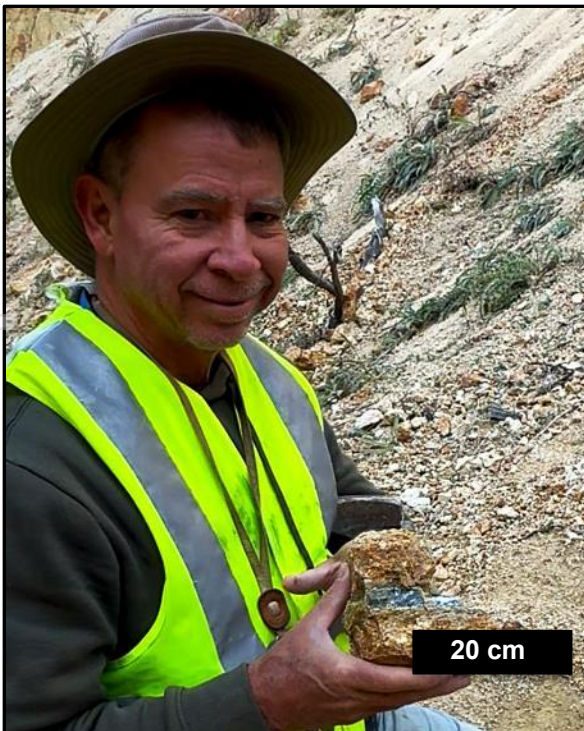
Figure 3: A rock sample, collected from a historical trench located at the Antimony Ridge Target, shows an example of sample material destined for metallurgical assessment. The rock sample exhibits a vein bearing a crystalline, grey-silver coloured metallic mineral stibnite containing between an estimated 20% and 30% stibnite. Stibnite is an antimony sulphide ore mineral, containing 71.7% mol weight antimony. Visual estimates potentially provide no information regarding impurities or deleterious physical properties relevant to valuations. A sample (Rock chip sample 329015) similar to this photographed rock specimen graded 19.15% antimony, 70.5g/t silver with 4.65g/t gold over 1m (see Resolution News Release of 11 June 2025, Figure 6 and Appendix C “Agreement To Acquire Major Drill-Ready Antimony-Gold-Tungsten Project In Stibnite Mining District, Idaho, USA”).
