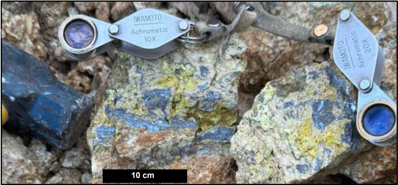
Figure 2: An example of sample material destined for metallurgical assessment. This rock sample, collected from a historical trench located at the Antimony Ridge Target, shows two rock specimens comprising the grey-silver coloured metallic mineral stibnite. Stibnite is an antimony sulphide ore mineral, containing 71.7% mol weight antimony. The stibnite in this rock specimen is crystalline in veins and brecciated veins, containing between an estimated 25% and 35% stibnite. Visual estimates potentially provide no information regarding impurities or deleterious physical properties relevant to valuations. A sample similar to this photographed rock specimen graded 49.8% Sb and 1,420 g/t Ag and 3.12 g/t Au (see Resolution News Release dated September 15, 2025).
