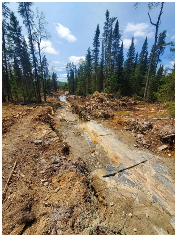
Figure 4: Sugar South stripping and channel sampling of outcropping vein
