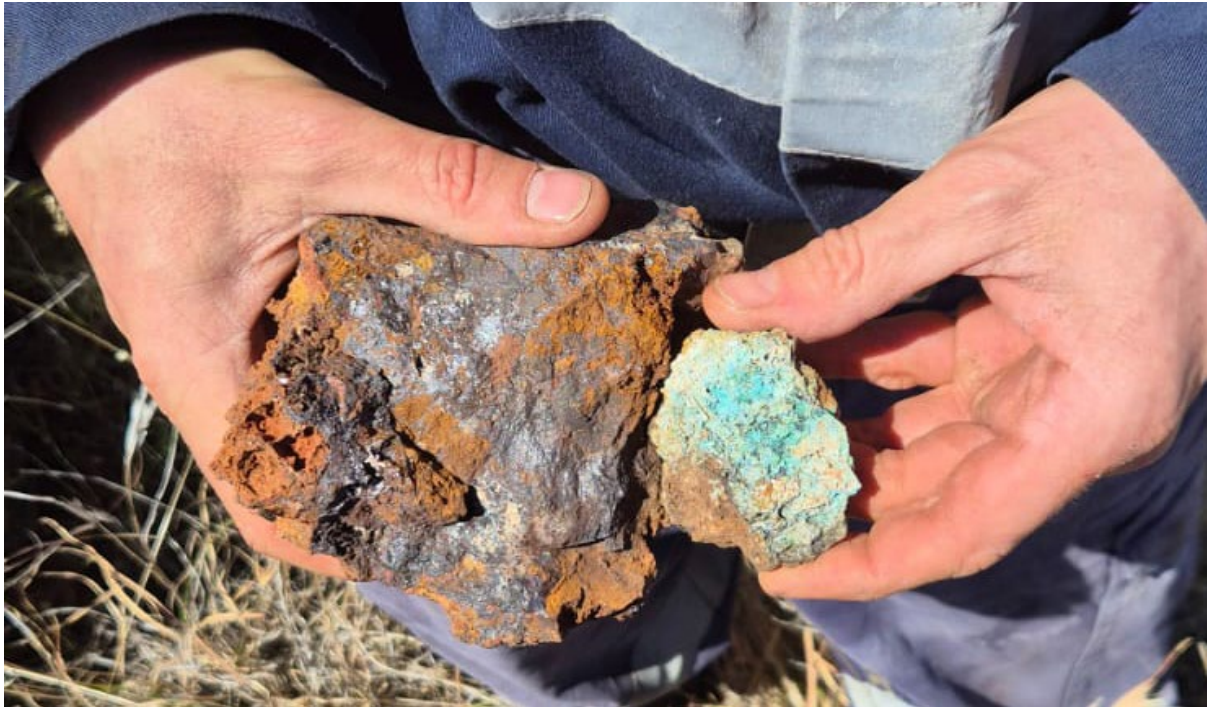
Figure 2. Gossan outcrop (482389E, 7438704N) showing classic ex-sulphide boxwork texture identified at VT1 immediately along strike from outcropping Oonagalabi Formation marble with oxidised copper mineralisation present.
