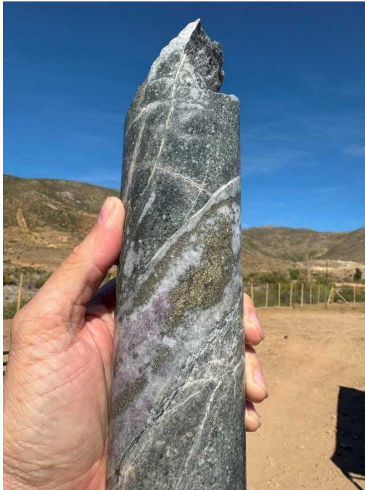
Photo 3 Anhydrite-pyrite-quartz vein within altered porphyry in 25LLDD0070 from 640m*.
